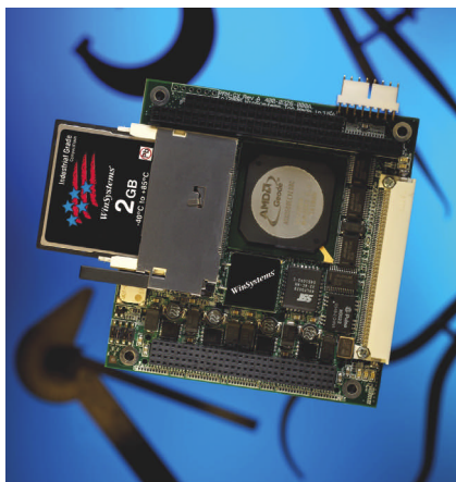
The low-power, 500-MHz, PPM-GX single-board computer features video, Ethernet, USB, and four COM channels; it operates from -40 to +85°C.
