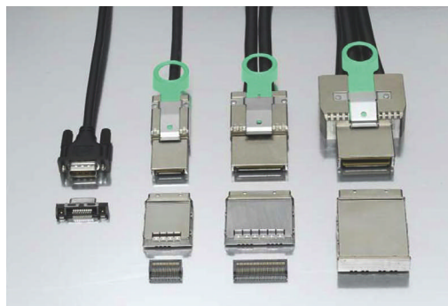
You can extend the PCIe bus outside the box using cables, a practice that the PCISIG recently standardized (courtesy Molex).
