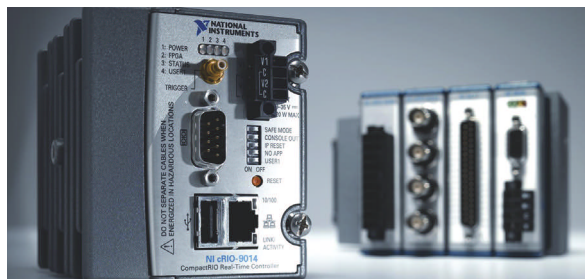
The new cRIO-9014 CompactRIO controller delivers increased processing speed, memory, and storage for high-performance embedded-control and -monitoring applications.
